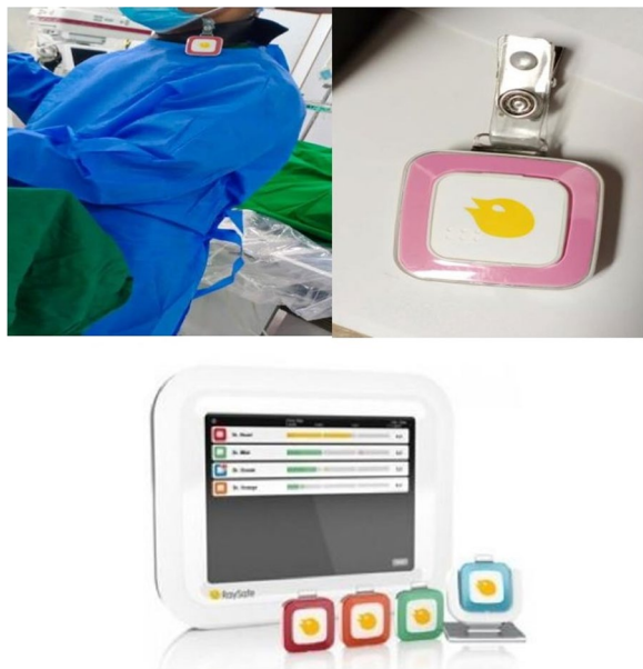
Fig. 2 Clockwise from above right: Dosimeter badge worn by staff above lead apron, below: badge placed in cradle connected to monitor to obtain effective dose value
